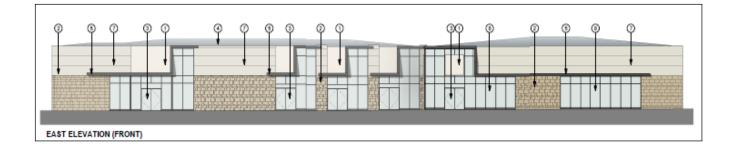
The schedule of materials for these units includes horizontal metal cladding above a stone effect cladding at lower levels for the walls of the buildings, powder coated frames for doors and windows and a composite roof panel arrangement.
